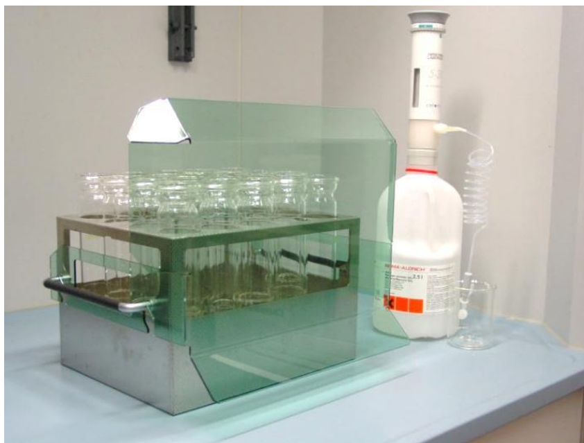
Figure 1: Safety accessories for the digestion with hydrogen peroxide and Kjeldahl Tablet Titanium
