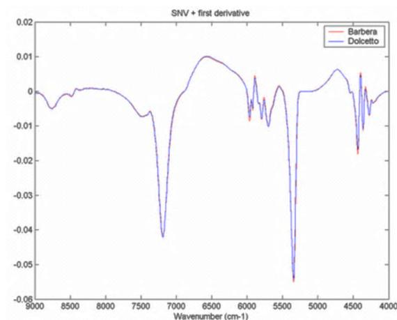
Figure 3: NIR spectra pretreated with SNV and 1st derivative.
