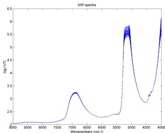
Figure 2: raw NIR spectra of red wine samples analysed
