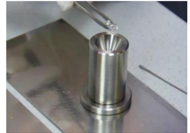
Figure 2: Manual pressing tool for tin foil packed samples.
