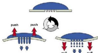
Figure 2: Droplet generation with the Nano Spray Dryer B-90 HP.
