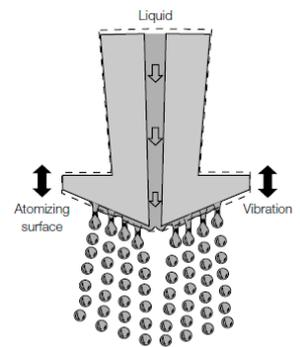
Figure 3: Ultrasonic nozzle for Mini Spray Dryer B-290.
