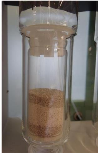
Figure 1: Twisselmann extraction chamber before start
