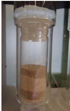
Figure 1: Twisselmann extraction chamber with sample before start
