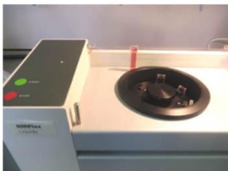
Figure 2: NIRFlex N-500 Liquid Cell for measurement of alcohol content in transmission mode
