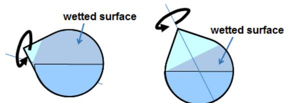
**Figure 2:** Representation of the wetted surface of an evaporating flask. A flatter immersion angle results in a larger wetted surface area inside the flask (left); a steeper immersion angle results in a smaller wetted surface area inside the flask (right).
