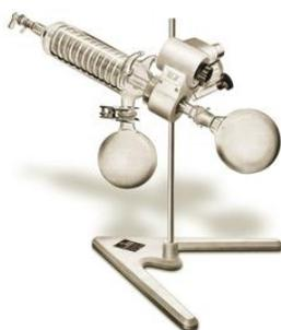
**Figure 1:** First generation rotary evaporator (BUCHI Rotavapor, Model 1957).
