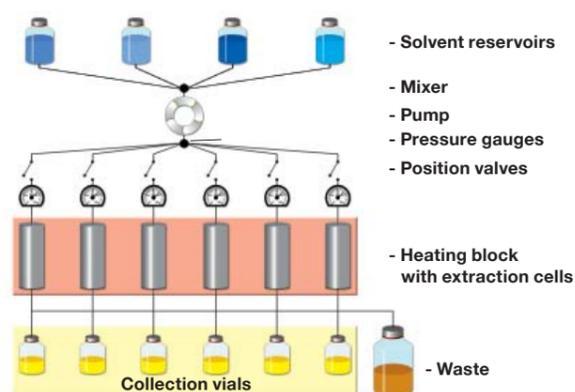
Fig. 1: Schematic representation of the SpeedExtractor E-916 set-up
