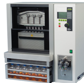
Fig. 2: SpeedExtractor E-916 for parallel pressurized solvent extraction (PSE) of 6 samples.
