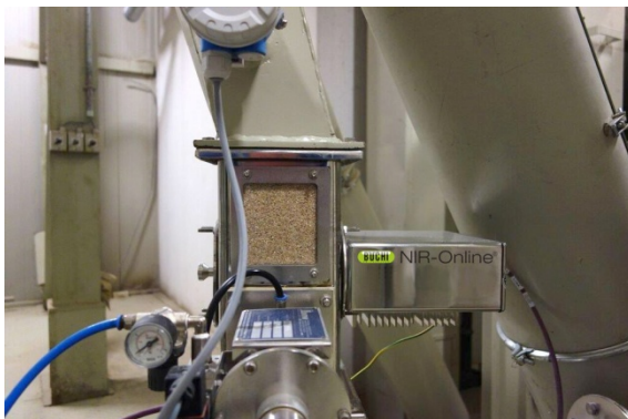
Figure 4: the NIR-Online sensor ensures timely control of the mixing and pelleting processes.
