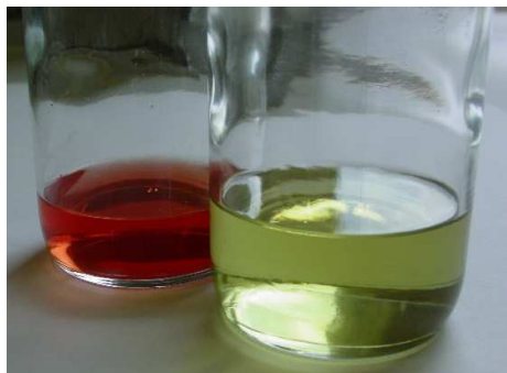
Figure 3: Colored extracts of pre-extraction (green) containing chlorophyll and of the main extraction (red) containing the hypericin
