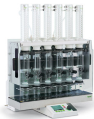
Extraction Unit E-816 SOX & HE 지방 추출
