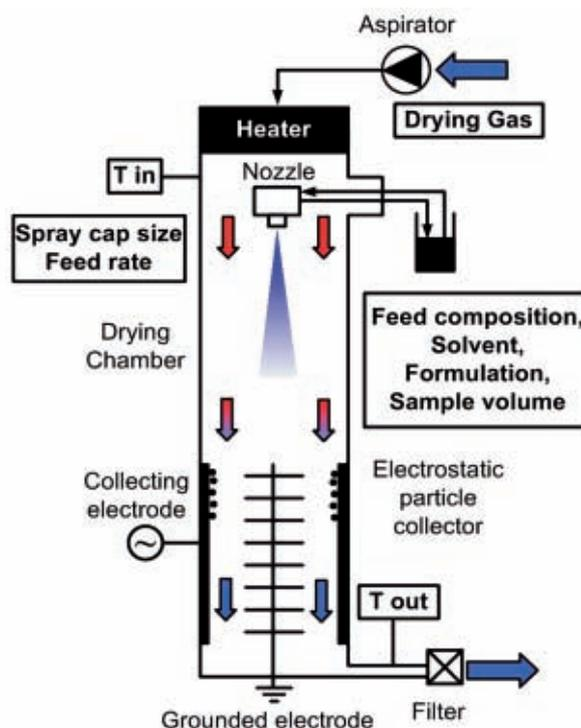
Fig. 3. Principle of the Nano Spray Dryer B-90 [8]
