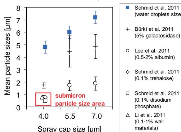
Fig. 4. Correlation between droplet and particle size (data from literature). The submicron particle size area is typically reached when using the 4.0  $\mu\text{m}$  spray cap and diluted solid concentrations of about 0.1 w%.
