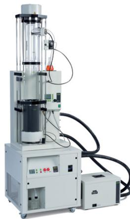
Figure 7 – Nano spray dryer B-90 in combination with the inert loop B-295
