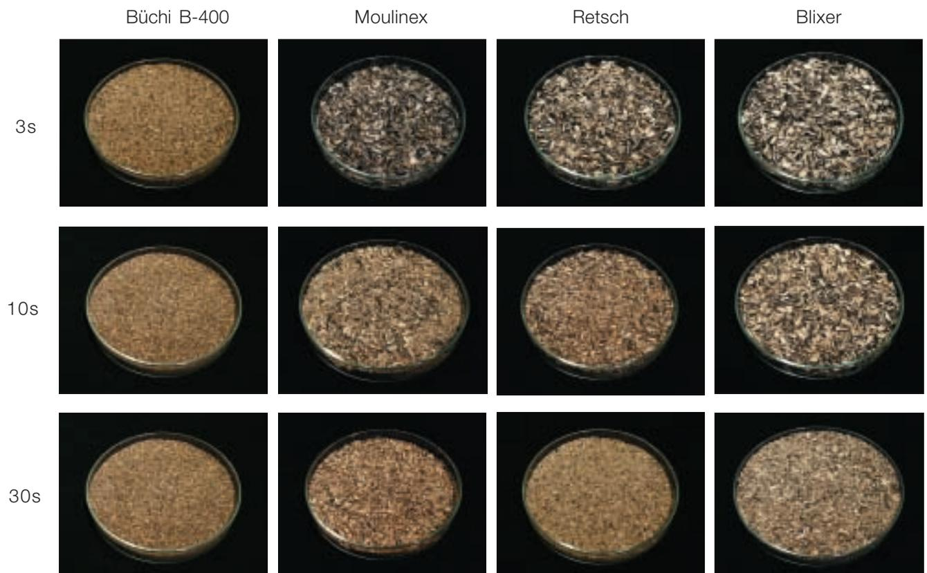
Fig. 1 Sunflower Seeds. Pictures taken after 3, 10 and 30 seconds mixing with Büchi B-400, Moulinex, Retsch and Blixer.
