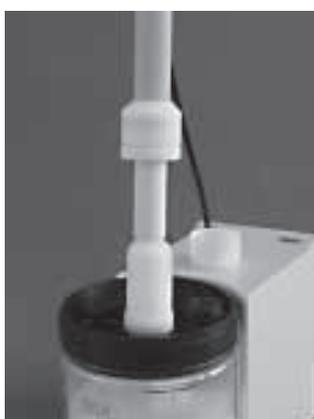
Now screw the cartridge with the side of the frit into the cartridge holder until the stop. Movement of the frit is prevented by the stop. For short cartridges of 75 mm length use the elongation.
