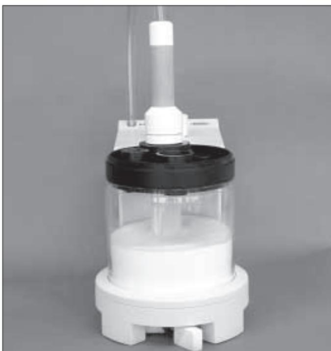
Submerge the cartridge into the fluidized gel. Open the valve on the front side of the cartridge. The cartridge is filled all at once. Leave the valve open and carefully withdraw the cartridge from the glass vessel.
