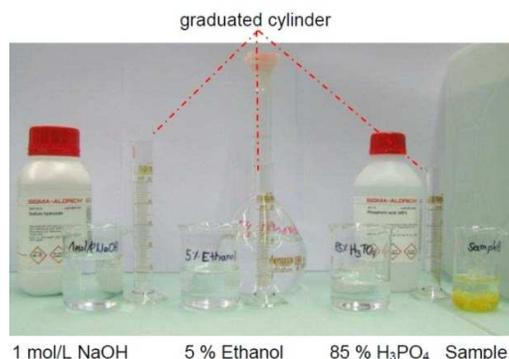
Figure 2: Chemicals required for preparation of solid samples
