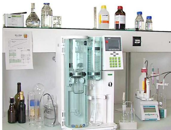
Figure 1: Setup for SO<sub>2</sub> determination
