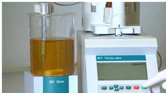
Figure 6: Titration setup with Pt-electrode
