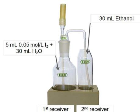
Figure 4: SO<sub>2</sub> absorption vessel
