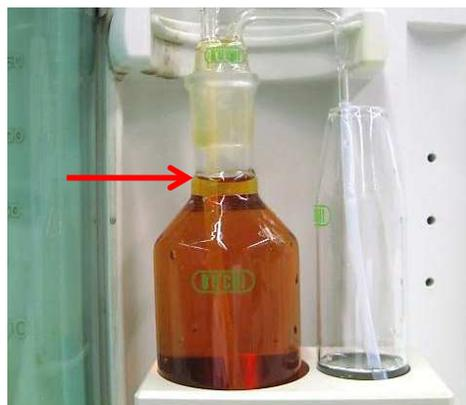
Figure 5: 1<sup>st</sup> receiver filled with distillate to the bottle neck
