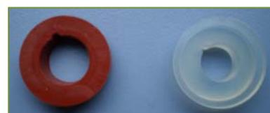
Figure 9. O-Ring Appendix insulation for Analyst sample vessels. Left: for 1ml Appendix; Right: for 0.3 ml Appendix.
