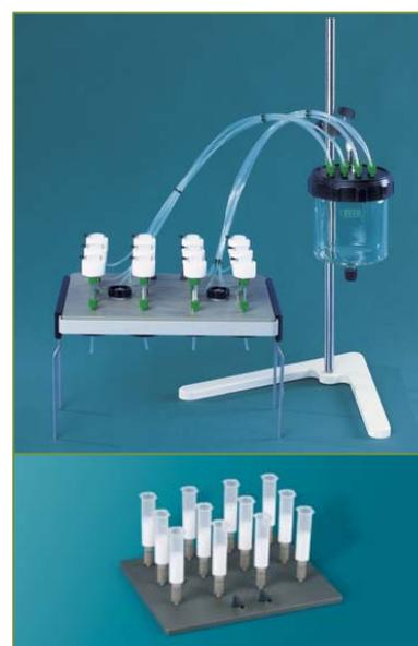
**Figure 4.** Above: SPE advanced module. Below: SPE basic module with equipped with 12 cartridges.
