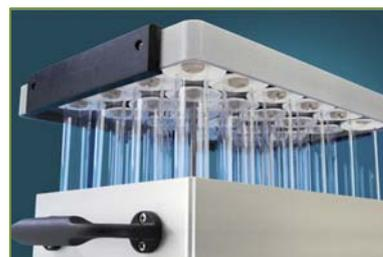
**Figure 2.** Exchangeable Polyvap rack with 24 sample glasses and a vacuum cover.
