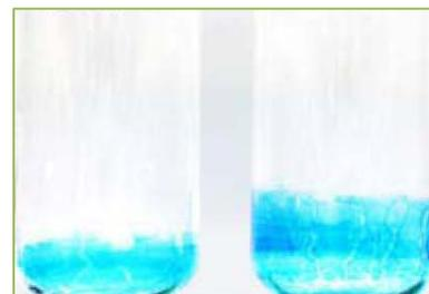
**Figure 17.** Grease sticking to the glass. Left after evaporation at 170 rpm (left) and 300 rpm (right).
