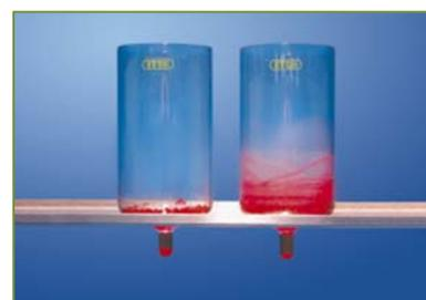
Figure 11. Effect of the Flushback Module. Left: When using the Flushback Module the analyte is collected in the appendix. Right: Without using the Flushback Module some analyte sticks to the glass wall of the vessels.
