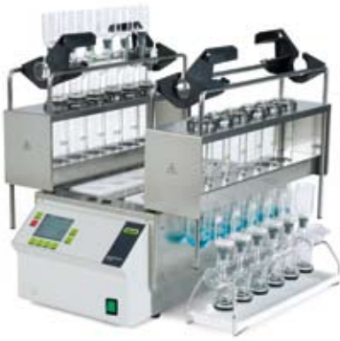
Picture 3: SpeedDigester K-439 with H 2 O 2 suction module
