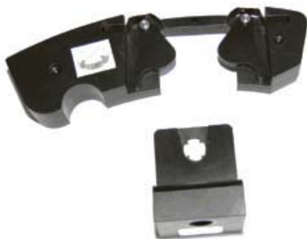
Fig. 6: Format-specific cups with two clamps (open and closed)
