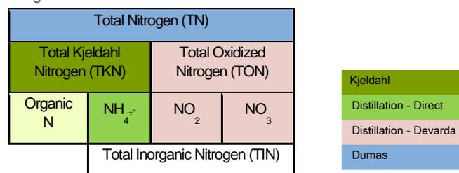
Figure 1: Nitrogen compounds which can be analyzed with the two methods Kjeldahl and DuMaster.
