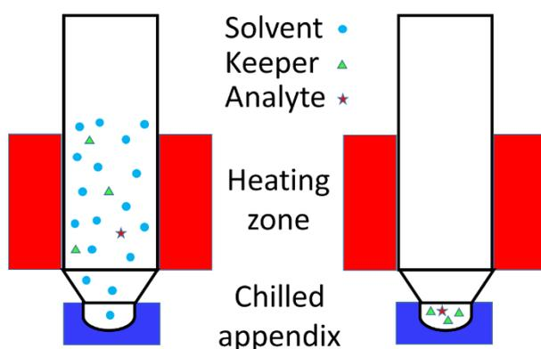
Figure 1: Functional principle of a keeper solvent: while the main solvent is evaporated, the analyte and the keeper are retained in the chilled appendix.
