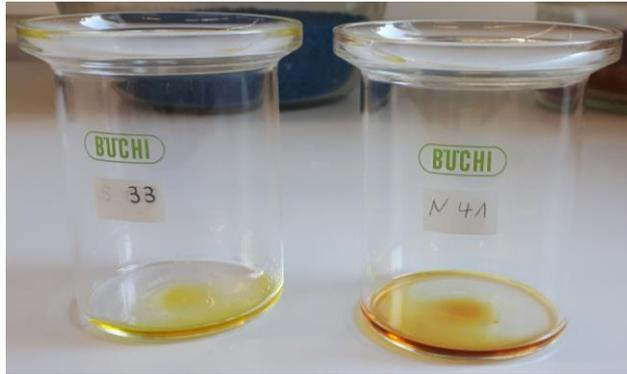
Figure 2. Extracted fat without hydrolysis (left) and with hydrolysis (right). The color of the hydrolyzed sample has changed to brownish, which can indicate a change in the fat quality.
