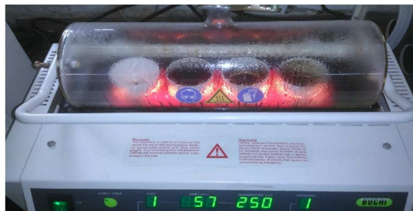
Figure 1. Digestion and ashing using the Wet Digester B-440.
